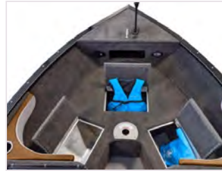
Remove the bow cushions to reveal an aerated 19 US GAL livewell and tons of storage.
